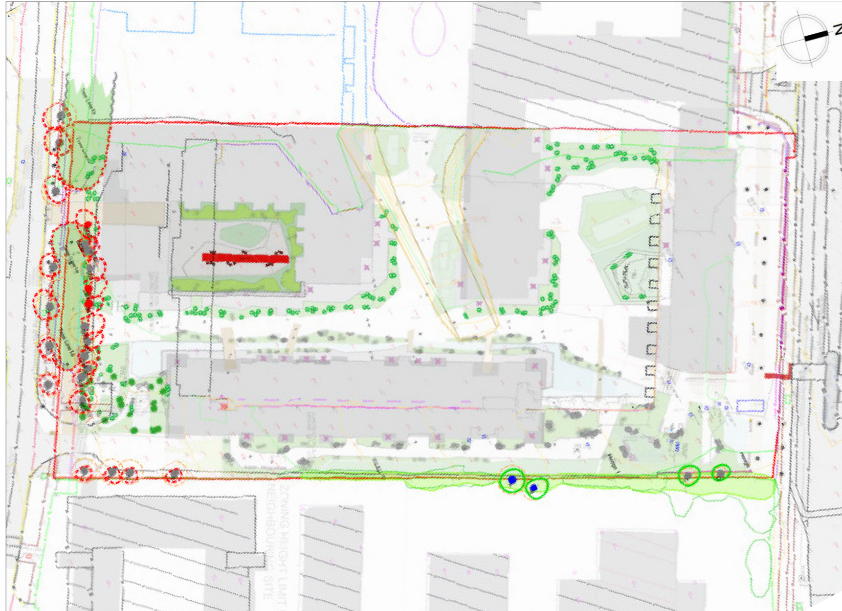
Figure 7: Extract from the Tree Impact Plan prepared by Andy Worsnop of 'The Tree File'
